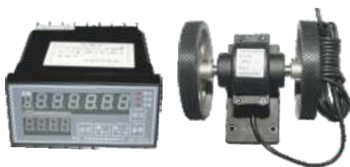
计长仪 Length measuring instrument
